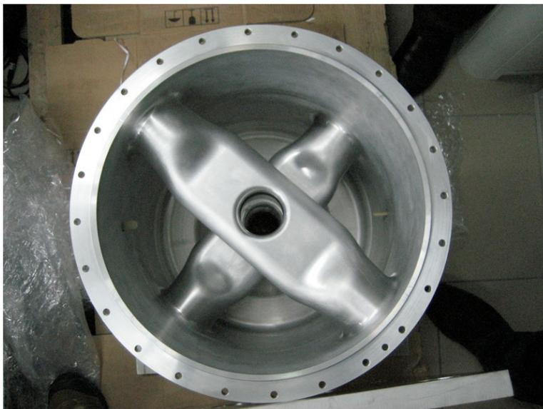
**Figure 5.** Double-spoke resonator cold model.
